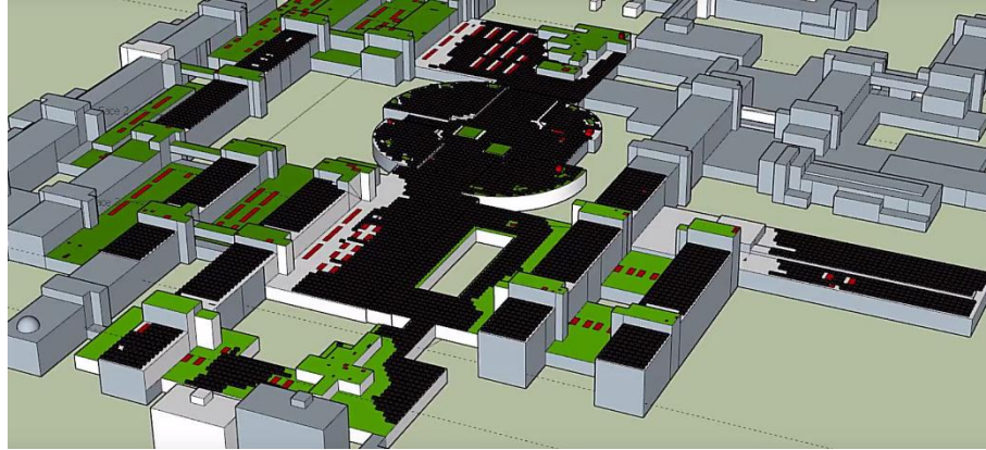
Concept plan of the 2.2 MWp PV array on the rooftop of University of Oulu Linnanmaa campus
